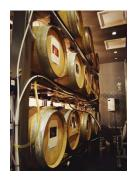
**AC Distributing** showcased their new Rack AeriAle direct barrel draw system. This hybrid-design, draft beer dispensing system utilizes technology from the original beer dispensing system to bring barrel-aged beers from the barrel directly to the tap system through EJ Beverage Ultra Barrier tubing.
